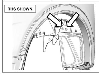
Punch out the cores of both black rivets located in the front of <u>both</u> rear wheel arches, using a Ø3mm pin punch & hammer.
