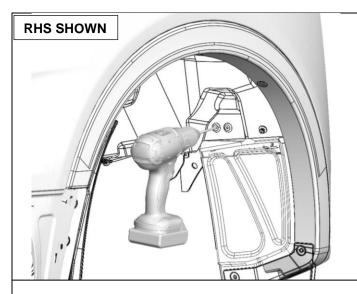
3. Drill out the remainder of the rivets with a Ø6.5mm drill bit.
