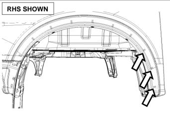
6. Carefully peel the front of the wheel arch flare back far enough to access the two M6 fasteners behind. Clip positions shown.
