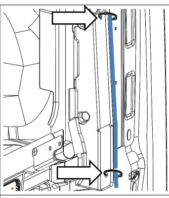
23. On the RHS only, secure wiring harness to the outside face of the J brace using the cable ties supplied.
