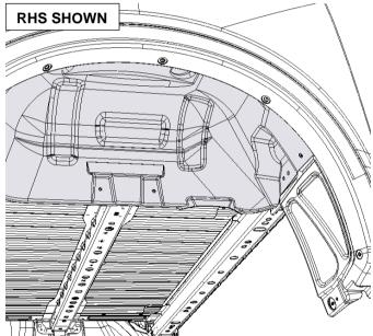
24. Reassemble wheel arch liner, flare and mouldings following steps 4-10 in reverse order. Replace any damaged clips or scrivets.
