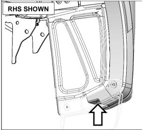
5. Remove the M6 fastener from the lower wheel arch moulding.
