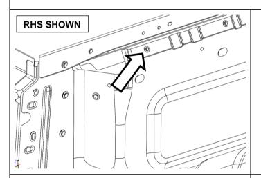
26. Locate the captive nut in each front corner of the tub.
