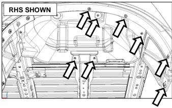
4. Remove 8 scrivets from the front half of each wheel arch liner by undoing the middle screw.
