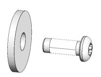
27. Assemble one M6x16 Pan Head Screw and 25mm OD Washer into the captive nut identified in the previous step. Repeat on opposite side.
