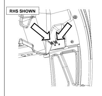
25. Install new rivets with M6x18x3 Flat washer under the head of the rivet.
