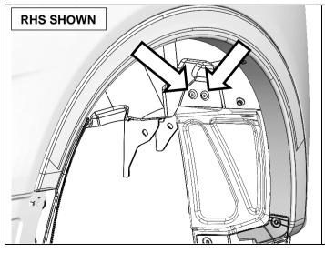
2. Punch out the cores of both black rivets located in the front of <u>both</u> rear wheel arches, using a Ø3mm pin punch & hammer.
