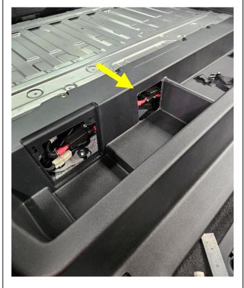
48. Reinstall the plastic trim and floor carpet, ensuring all fasteners are properly secured. Installation is reversal of removal procedure.
