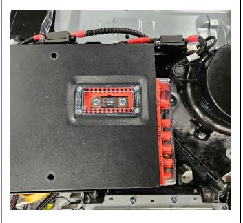
39. Install the four Bolts M8x65mm and Washers M8 through the battery holes into the Mounting Bracket.
