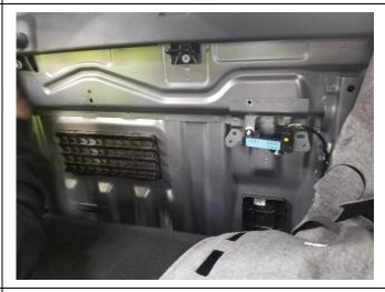
8. Remove the left hand child seat restraight. This fastening point is used to secure the Mounting Bracket.
