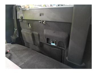
16. Cut fabric trim to gain access to rear cabin fastening points above the antenna.
