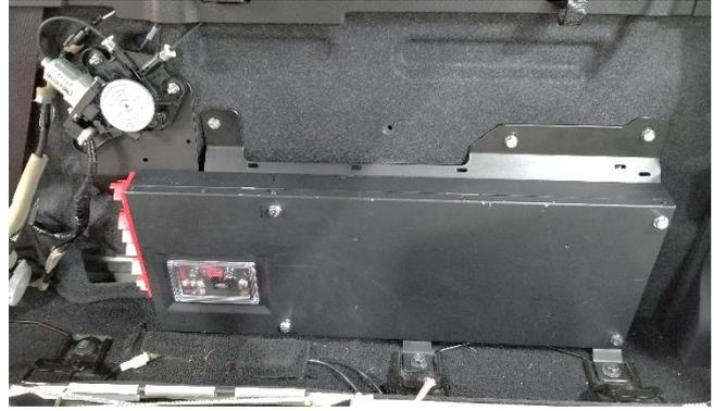
32. Ensure the slimline battery rocker switch is OFF before the harness installation.
