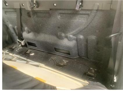
6. Pull upper plastic trim panel forward to disconnect all clips. The panel does not require complete removal, leave panel loose to allow fabric trim to be removed.
