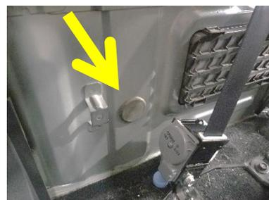
18. Remove retaining bolts from the passenger side lower seat support.
