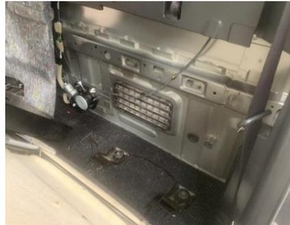
9. To install the Nutserts M8, drill out two existing holes on the crossmember as shown in images.
