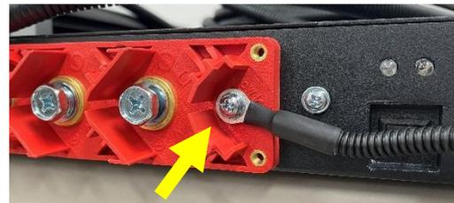
54. Reconnect the start battery positive (+) terminal, then the negative (-) terminal.
