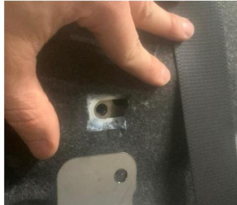
22. Install supplied Bolts M8x25mm and Washers M8 through two nutsert Mounting Bracket holes, install Spacers 4mm between Mounting Bracket and vehicle rear cabin wall.
