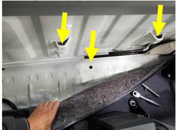
Five holes on vehicle cabin.
