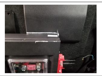
16. Remove battery and cut plastic trim along marked line.
