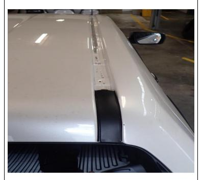
Remove channel trims from both sides, do not remove the rear most pieces.
