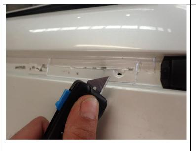
2. Locate the 8 (4 per side) captive nuts and using a safety knife, expose the holes.
