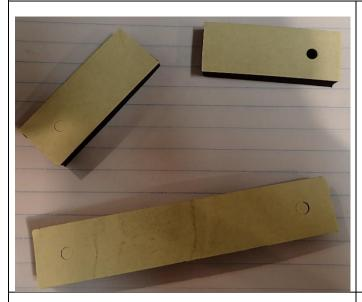
4. Cut Rubber packers in half and stick to the feet so that the holes line up
