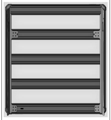
8. Flip the blade brackets over so they are upside down and carefully place on top of the BASE RACK. When doing so ensure the coach bolts in the stud plates go through the slots. Then secure the blade brackets to the BASE RACK using M8 flat washers and nyloc nuts.
