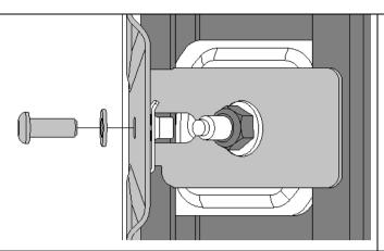
9. Secure each of the 4 mounting plates to the air deflector. Use the M6 Button head screws and black M6 washer (part# 4584329) as shown.
