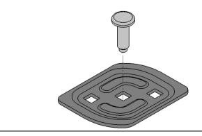
4. Insert one M8 x 25 Stud into each of the Stud Plates as shown.
