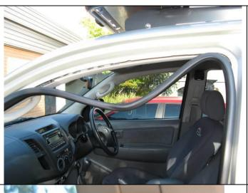
5. Pull down the door seals so the interior trim can be removed.
