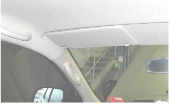
1. Remove the sun visors. Remove the SIX grab handles from the pillars.
