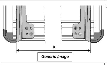
29. Using the previously recorded measurements, adjust the location of the blade bracket on the BASE RACK.
