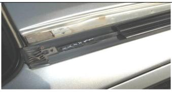
10.Remove the exterior roof trim from both sides of the vehicle. Take care not to bend the trim, as it will be reused.
