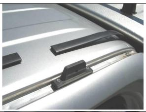
21. Cut the roof trim that was removed earlier at step 10 to fit neatly around the roof rack mounting blocks. There will be six pieces in total for both sides of the roof.
