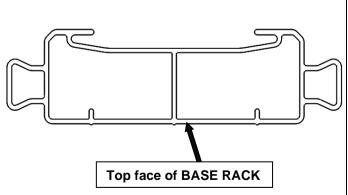
24. Place the BASE RACK face down on a clean flat surface. Provide protection to the top face of BASE RACK to avoid marking of surfaces
