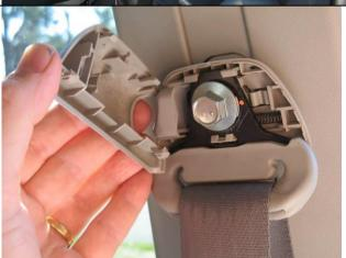
6. Remove the front and rear top seatbelt mounts.
