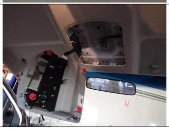
4. Carefully remove centre roof console and unplug.
