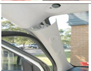
7. Remove the plastic trim from the front, middle and rear pillars on each side of the vehicle. They can simply be pulled away to be released from their mounting clips.
