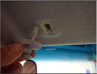
2. Remove the plugs located around the periphery of the ceiling. They are located at the front at the driver's side, the rear of the ceiling at the right & left side of the vehicle and above the rear windscreen.
