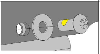
33. Use the M8 Button head Torx screws and M8 Black washers to secure the BASE RACK to the roof mounting brackets.
