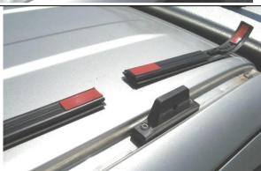
22. The fitting kit includes two pieces of double-sided tape to be cut into equal lengths of 50mm (12 pieces). Apply tape to each end of the roof trim pieces and stick the roof trim back in place by following steps 1 – 8 in reverse order.
