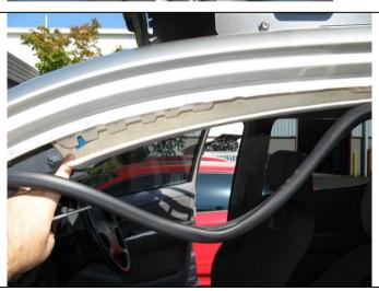
8. Carefully lower the headlining as shown in the adjacent diagram. It does not need to be totally removed.
