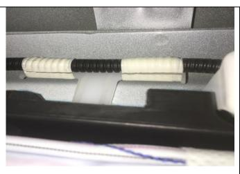
9. Once you can gain access behind the liner roughly gauge where the <u>rear</u> mounting feet will be located (explained in step 11). The tape holding spiral tubing will need to be cut in order for it to be moved out of the way so it is not damaged whilst drilling and during the installation. Once the installation is complete this can be reattached using tape.
