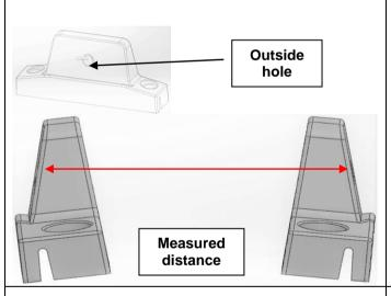
23. Using a tape measure, measure across the vehicle between the middle of the hole on the outside face of the front and rear set of mounting brackets. Make a note of each measurement.
