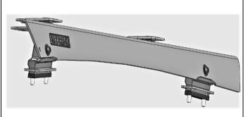
31. With assistance, carefully place the BASE RACK on the vehicle so the inside of the blade brackets rests on the outside of the mounting blocks. The entire BASE RACK assembly should be clear of the vehicle roof. All mounting holes/slots should align closely.
